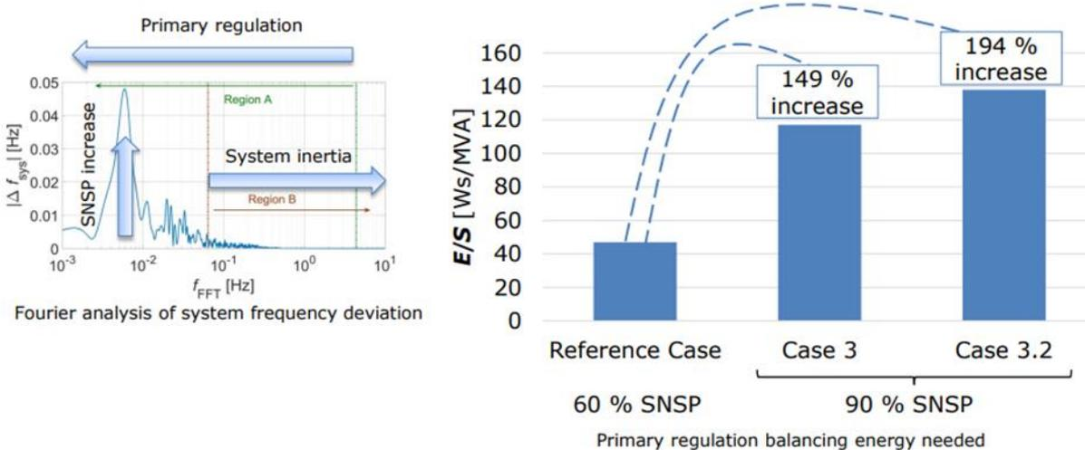
Fig. 3.3 Learning of the project Migrate from Ireland network study, request of primary regulation when System Non-Synchronous Penetration (SNSP) increases from 60% to 90% [3.18].
