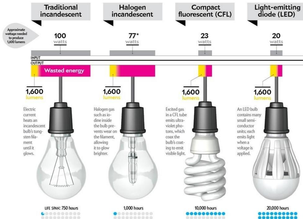
Fig. 6.2: Lighting systems: efficiency and longevity [6.12]
