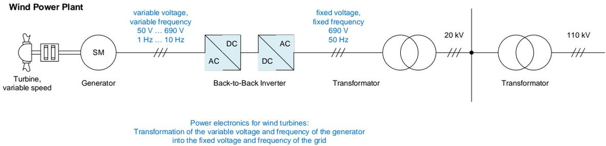
Fig. 2.6: Wind power plant based on synchronous generator and back-to-back power electronics inverter technology, enabling full control of power infeed to the electric grid electronics
