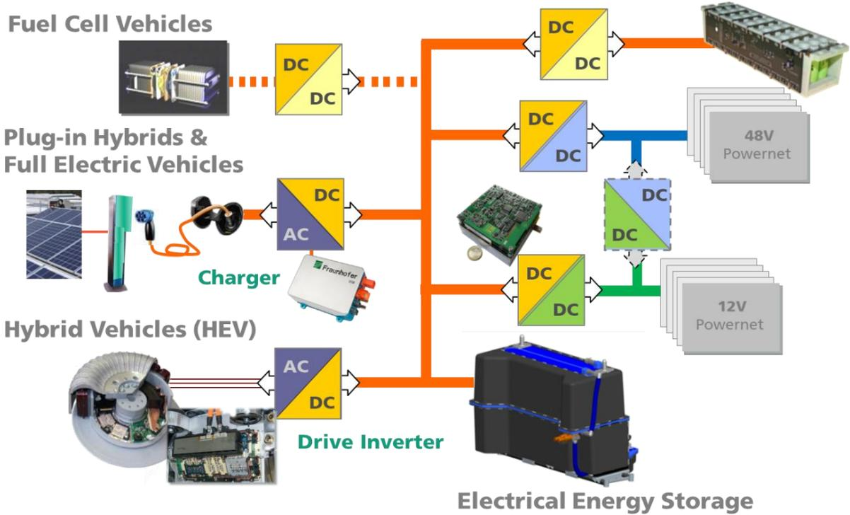
Fig. 4.2: Power train of electrified cars (hybrid, full-electric or fuel cell vehicles), electronics
