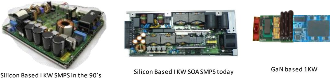
Silicon based design reaches a point of Maturity improvement of one attribute is usually at the cost of another Manufacturing is labor intensive EMI is treated a mix of science and art
