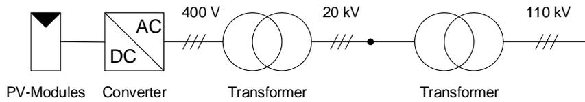
Fig. 2.7: Basic structure of a solar power plant with power electronics inverter to convert dc to ac power, enabling full control of power infeed to the electric grid electronics
