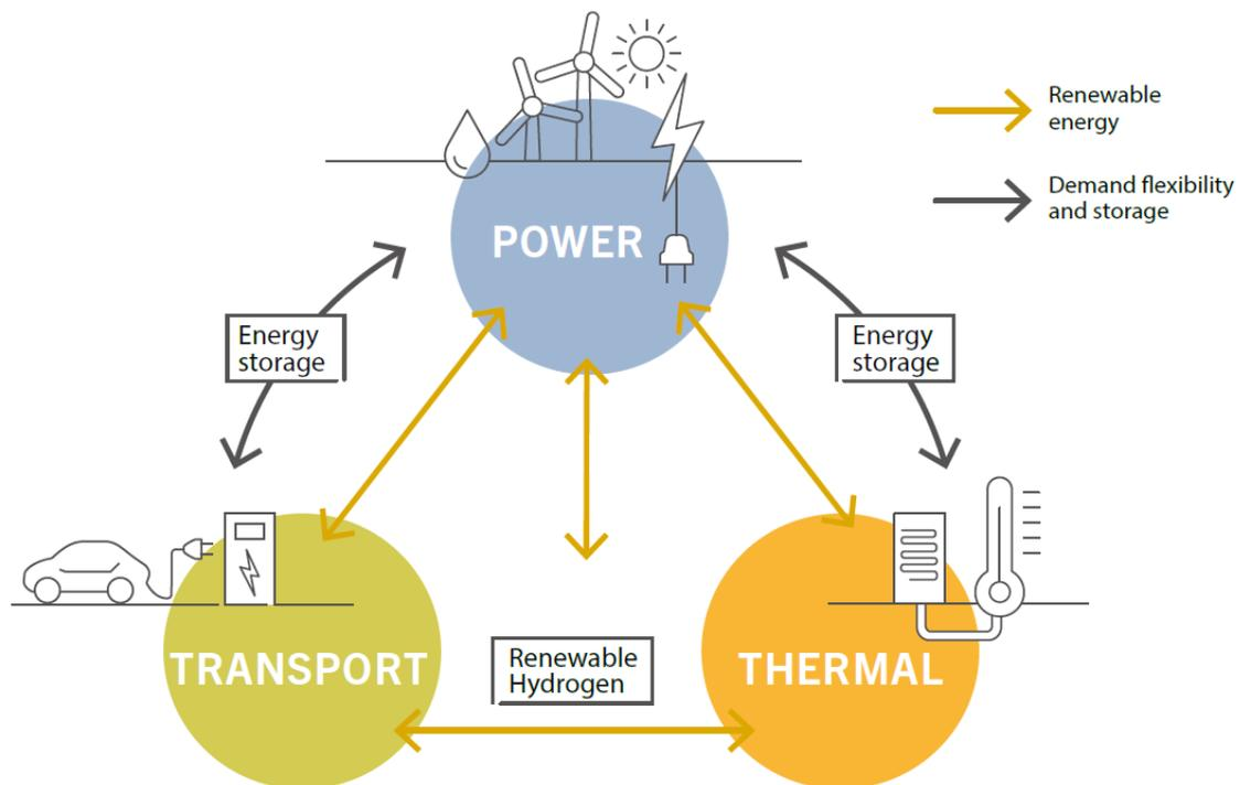
Fig. 2.1: Coupling of power, thermal and transport sectors, [2.4], p. 204
