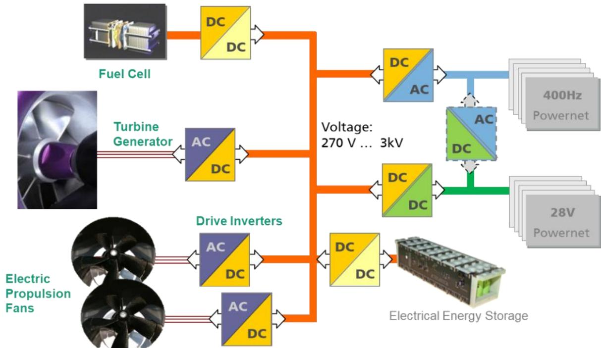
Fig. 4.5: Future electric power train of electric propelled aircrafts
