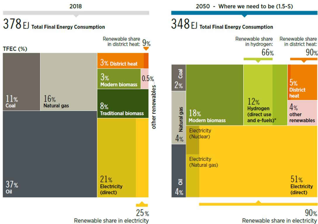
Fig. 2.2: Breakdown of the total final energy consumption (TFEC) by energy carrier: the share of electricity is supposed to increase from 21% in 2018 to 51% in 2050, with a total renewables share of 90%, in order to reach the 1.5°C goal by 2050 ([2.3], p. 71)
