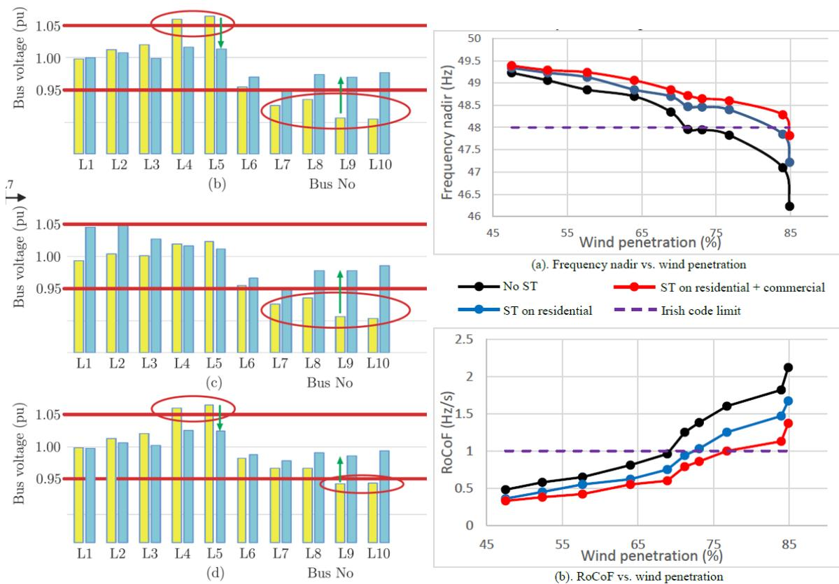
Fig. 3.2 Potential of Smart Transformers (ST) by meshing a distribution grid (a: yellow radial grid, blue with ST-meshing) [3.8] and by controlling voltage-sensitive loads (b: impact on Ireland-grid [3.13])
