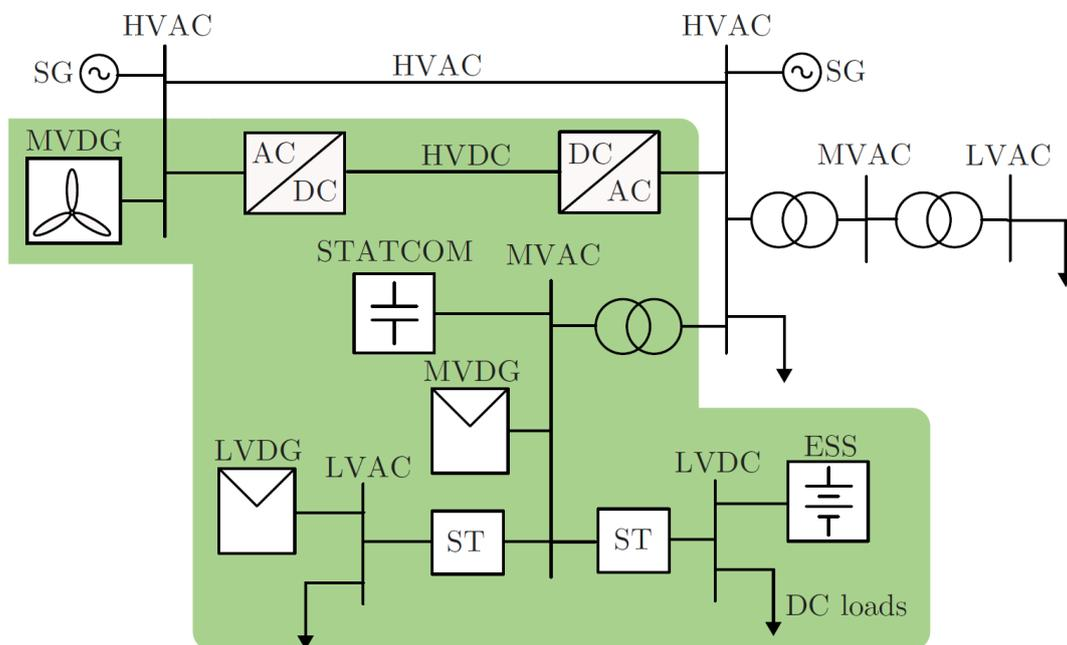
Fig. 3.1 Power electronics contributing to the future electronic grid systems.
