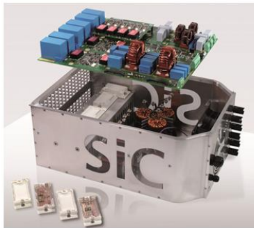
Generation 1 (2012) SiC JFETs, 48 kHz pulse frequency 18l - 18,4 kg (15kW) conventional packaging
