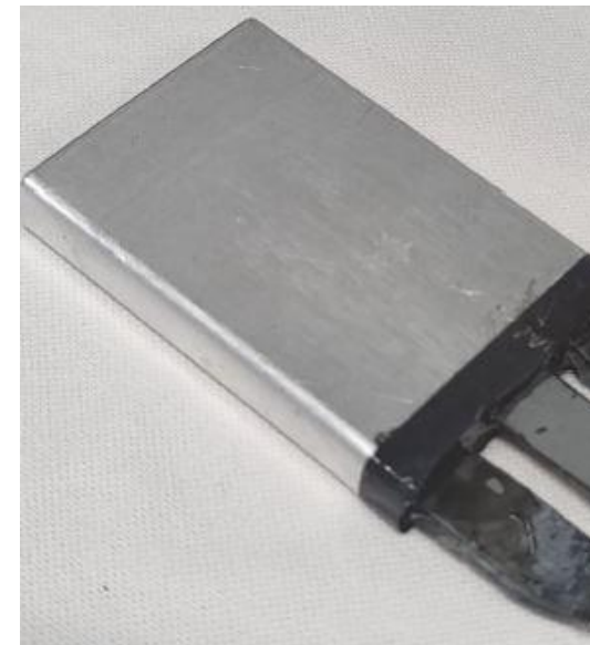
Left: Canned capacitor with 32 \mu F
