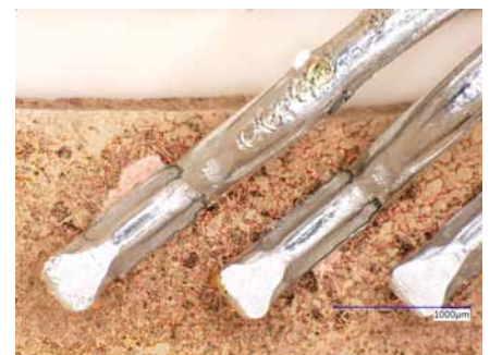
Corrosion due to mal Silicone gel adhesion in the area of Al bond wires
