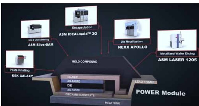
ASM supports various assembly process steps in the power module production.
