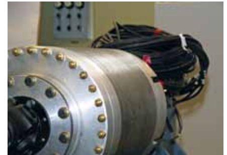
Fig.: 4000 Nm traction drive
