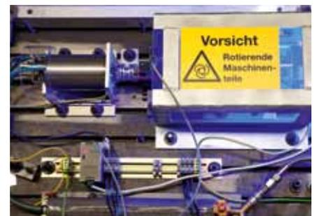
Test bench for a high speed drive
