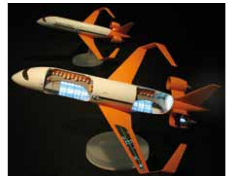
In 2012, Bauhaus Luftfahrt unveiled the pre-concept study "Ce-Liner" for a universally-electric short-to-medium range aircraft seating up to 189 passengers.
