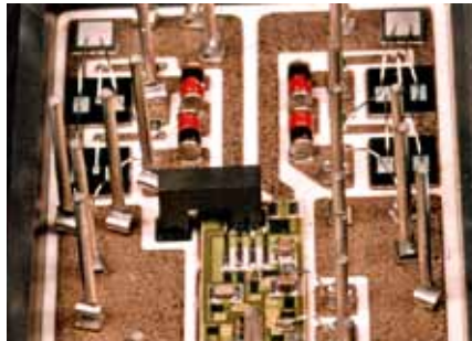
Power module for a fault tolerant drive
