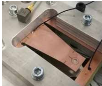
Demonstrator of PCB-based piezoelectric vibration energy harvester
