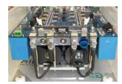
Highly efficient and compact three-phase fast battery charger (5kW/L with low-cost standard semiconductor devices within ECPE Project)
