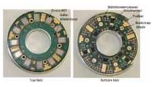
Multiphase inverter for direct integration in motor housing operating at 140°C ambient temperature
