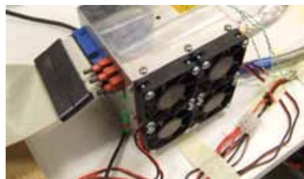
High power density (4kW/dm 3 ) inverter for 2.2 kW drive (95% efficiency) – ECPE project
