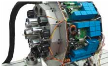
Fault-tolerant, high power density integrated machine and drive for aerospace applications (75 kW, 4 kW/dm 3 )
