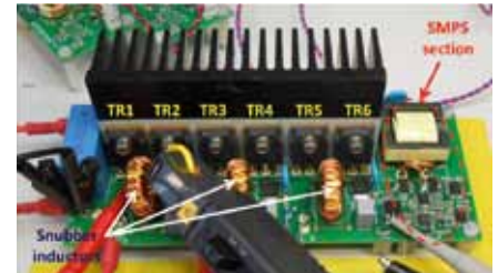
99% efficient three-phase inverter using super-junction devices.
