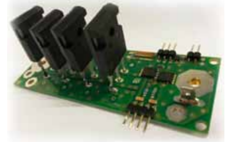
Fig.1 – Over current breaker based on the dual thyristor principle but realised with MOSFETs and a SiC JFET in cascode configuration
