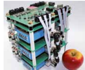
Full SiC boost converter (100 kW, 100 kHz)
