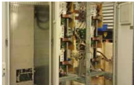
1 MVA power stack. IGBT modules.
