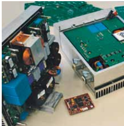
Bi-directional charger for electric vehicle, Smart-Wheels project
