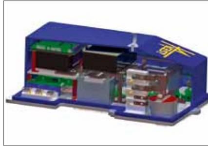
Integrated Power Unit (DC-DC converter and drive inverter) for hybrid electric vehicle, Europa-PlugIn project
