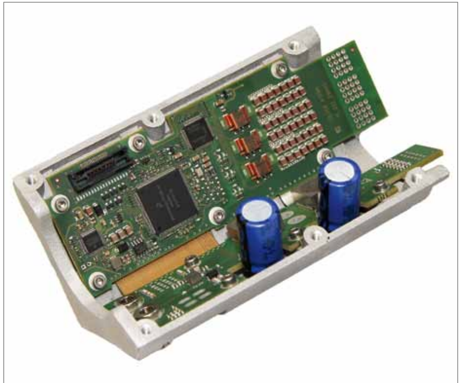
1.5 kW from 12 V: Control unit for an active roll stabiliser.
