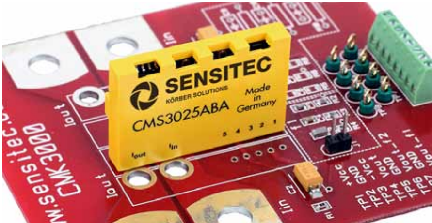
CMS3000 current sensor family for highly dynamic current measurement with up to 2 MHz bandwidth.
