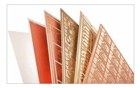
the copper. DBC (direct bond copper) – a high temperature melting and diffusion process where the pure copper is bonded
