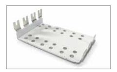
onto the ceramic and AMB (active metal brazing) – a high temperature process where the pure copper is brazed onto the ceramic substrate. The high heat conductivity of the ceramic as well as the high heat capacity and thermal spreading of the thick copper cladding makes curamik® substrates indispensable to power electronics.
