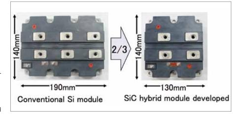
JBS structure successfully resulting in increased current per SiC-SBD surface unit area. Further, as the internal electric field of SiC is approximately 10 times that of Si, the optimal device edge structure was designed using device simulation to decrease the electric field around the device edge and assure the reliability required for rail cars.
