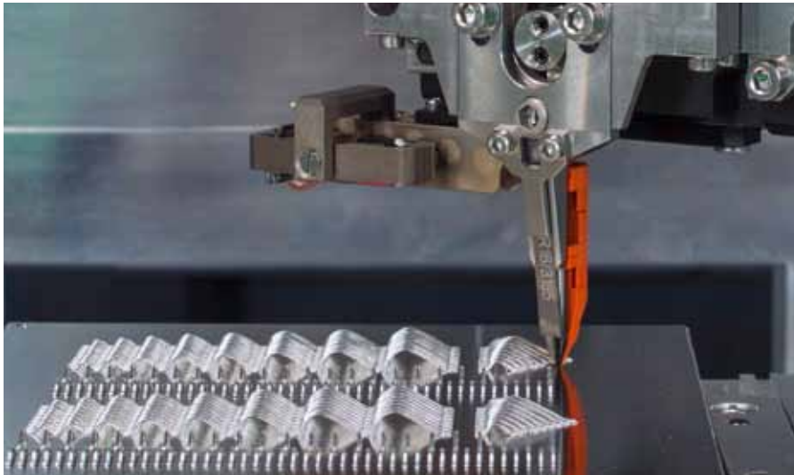
Heavy Wire bonding – detailed view
