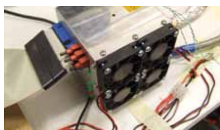
High power density (4kW/dm 3 ) inverter for 2.2 kW drive (95% efficiency) – ECPE project
