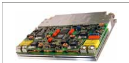
Ultra-efficient / compact automotive DC/DC converter; 99% @ 40kW/dm 3 .
