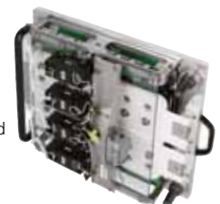
6.5kV-750A IGBTs based Half Bridge module
