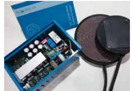
3kVA contactless battery charger
