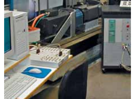
Test bench for sensorless operation of permanent-magnet synchronous motors including realtime development system, motors and converters.
