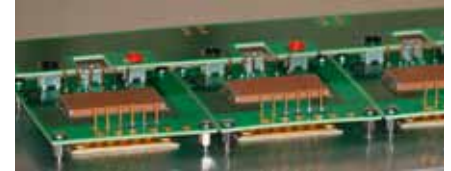
SiC-JFET based inverter for 300°C ambient temperature operation
