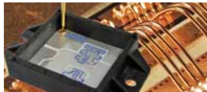
Thick-film based power module and copper wire bonds.
