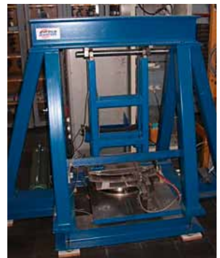
Test bench of slot less PM synchronous linear motor (drive for stratosphere-infra-red-telescope SOFIA)
