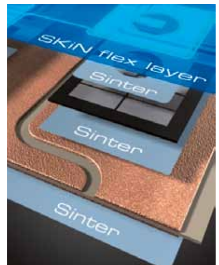
Wire bond-free packaging technology for power semiconductors
