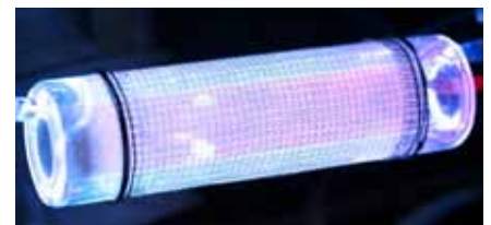
Laboratory sample of a pulse-driven Dielectric Barrier Discharge radiation source for disinfection purposes.
