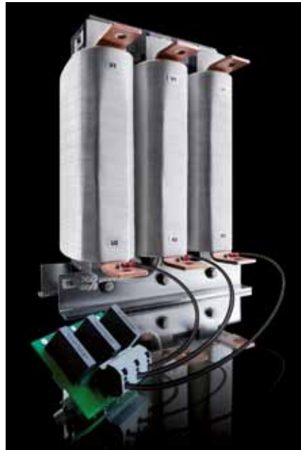
dU/dt output filter for reduction of voltage stress at motor windings, protecting AC motors from destructive effects of peak voltages.
