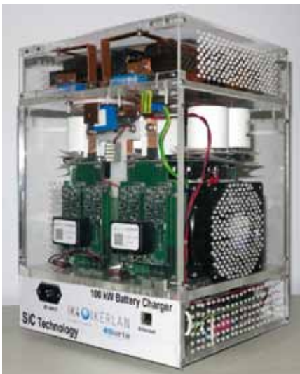
100kVA Full SiC converter
