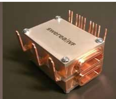
SiC packaging concept with double sided cooling and water jet formed vias
