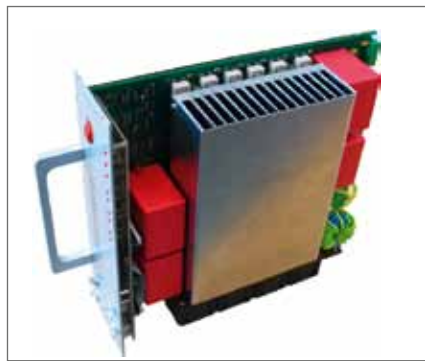
Single PCB converter (DC-Link voltage: 900V, max. output current: 130A, maximum power: 25kW)
