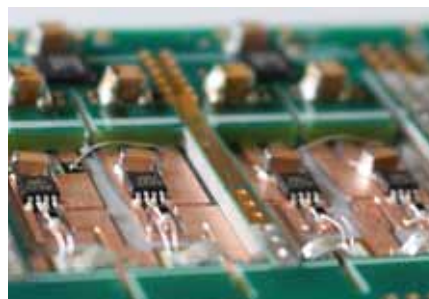
Multi-chip-module (MCM) soldered on a printed circuit board (PCB) for low-inductive connection of dc-link for fast-switching converters.
