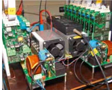
Power section with driver and filter circuits of an experimental converter
