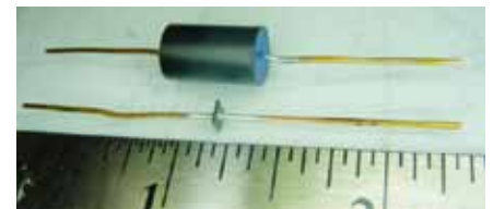
10 kV SiC PIN diode developed by Ascatron and Acree for Alstom Power
