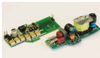
LED driver comparison. Left: DTU design. Right: Commercial product.
