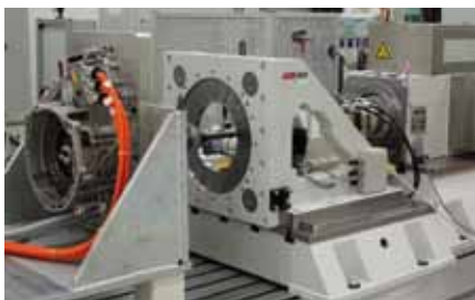
High speed motor test bench (up to 200 kW, 30.000 min -1 )
