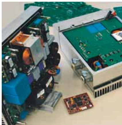
Bi-directional charger for electric vehicle, Smart-Wheels project
