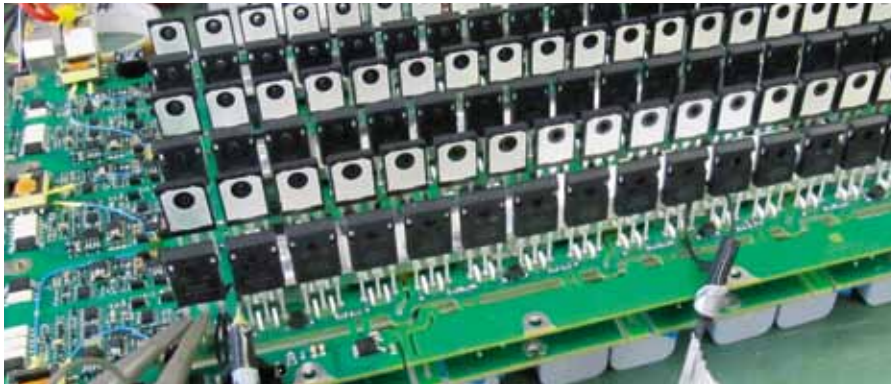
SiC MOSFETs in 750 V, 400 A inverter developed by Inmotion Technologies
