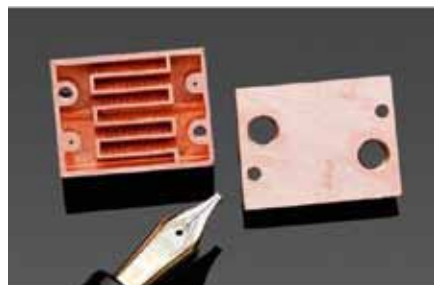
Direct manufacturing from powder of Cu cooler for SiC application
