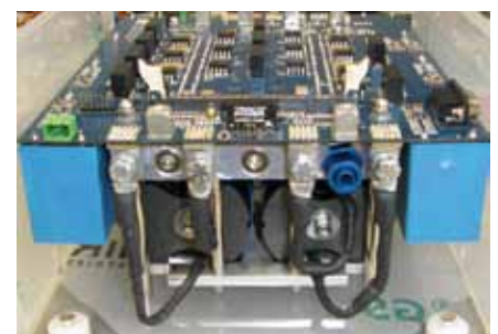
Highly efficient and compact three-phase fast battery charger (5kW/L with low-cost standard semiconductor devices within ECPE Project)
