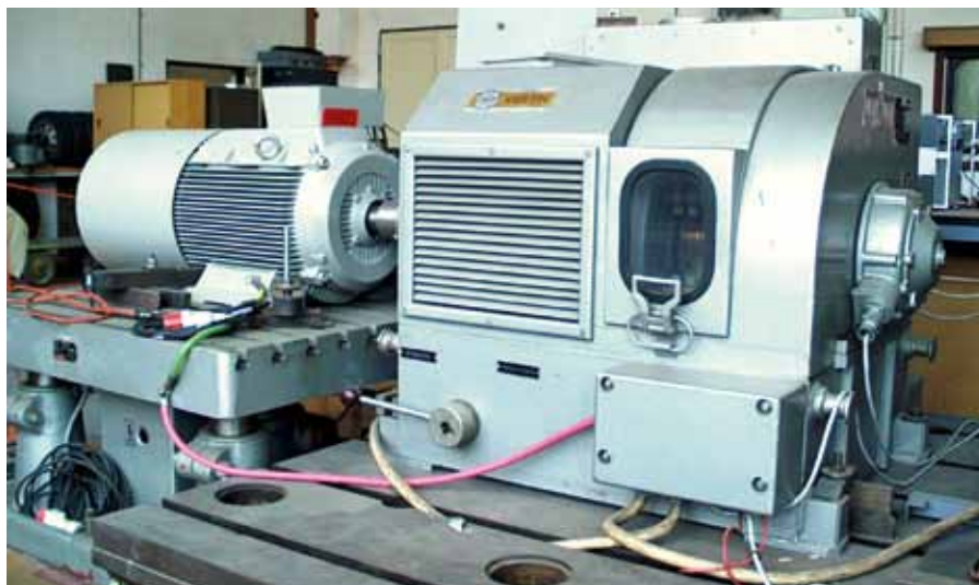
Dynamometer with rated power of 160 kW in Laboratory of Power Electronics
