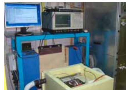
Fig. 2 – Non destructive tester for power semiconductor devices at temperature ranging from -50^{\circ}\text{C} up to 200^{\circ}\text{C} .
