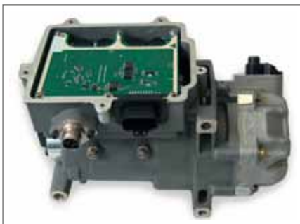
300 V converter for the precise control of a brushless DC motor
