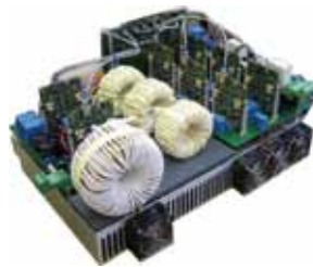
20 kW, 3-phase, bidirectional, isolated AC-DC converter based on SiC MOSFETs
