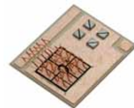
Conductive adhesives and copper wire bonding enable new interconnection technologies for power electronic applications
