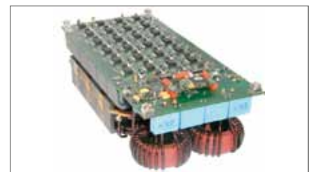
Ultra-high efficiency 3.3kW 1-ph. PFC rectifier; (efficiency at rated power: 99,4 %).
