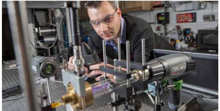
Spatial-resolved spectroscopy of novel microwave-driven mercury-free energy saving lamps.
