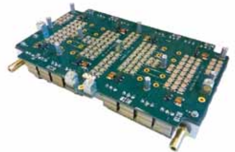
Liquid-cooled DC-DC-converter with very high power density
