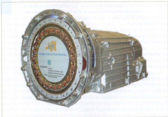
Figure 1: Electric drive with the power electronics, both integrated into the clutch-box screwed at the gear-box
