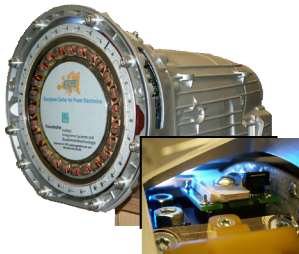
Fig. 4: Automotive demonstrator: integrated drive for hybrid traction
