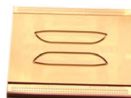
The Shi-Li chip design with microfluidic channels defined over four columns of silicon nanowires.
