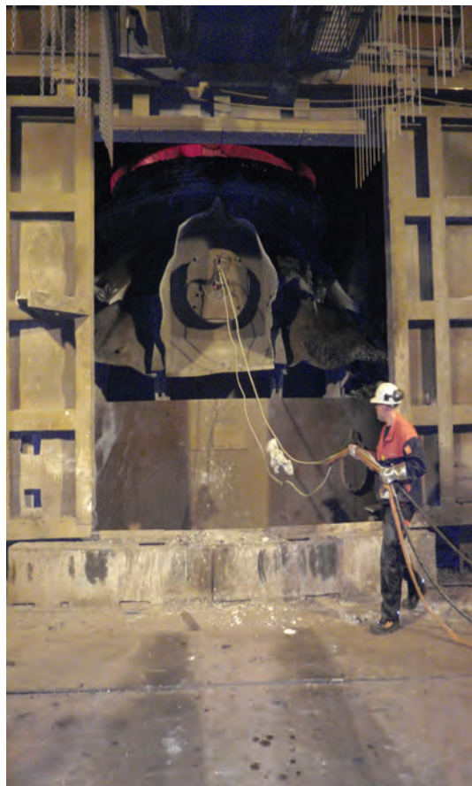
Fiber optic measurement in SSAB steel converter.
