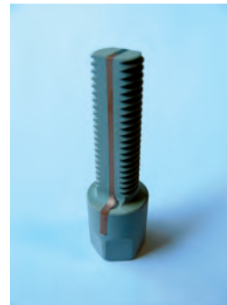
Industrial M10 bolt with a plasma electrolytic oxidized insulating layer and patterned Cu/CuNi wires from the bolts head to the top forming a thermocouple sensor structure.
