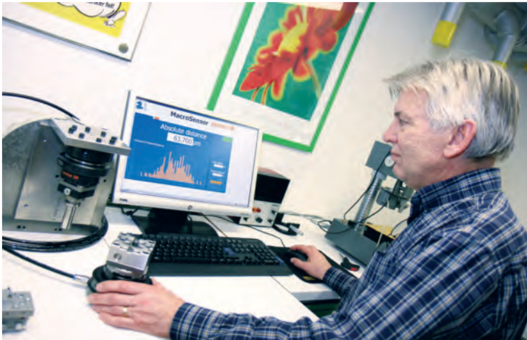
Fiber optic sensor system for nanopositioning. Photo used with kind permission from System 3R.
