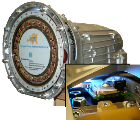
Fig. 4: Automotive demonstrator: integrated drive for hybrid traction
